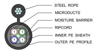
**PRODUCT DESCRIPTION**: Assembly of 4 microducts (m/d) to specification MHT 380, each with low friction performance for fibre blowing. The assembly is surrounded by a moisture barrier under a flexible polymer inner sheath. The flexible outer sheath 'figure-8' profile incorporates a steel strength member, and a defined web section between the steel and the tube bundle. Once separated from the strength member, the cable is metal-free.
